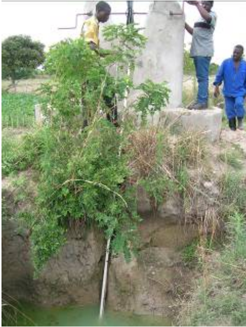
Figure 10: Rope pump extracting water from shallow well for irrigation
