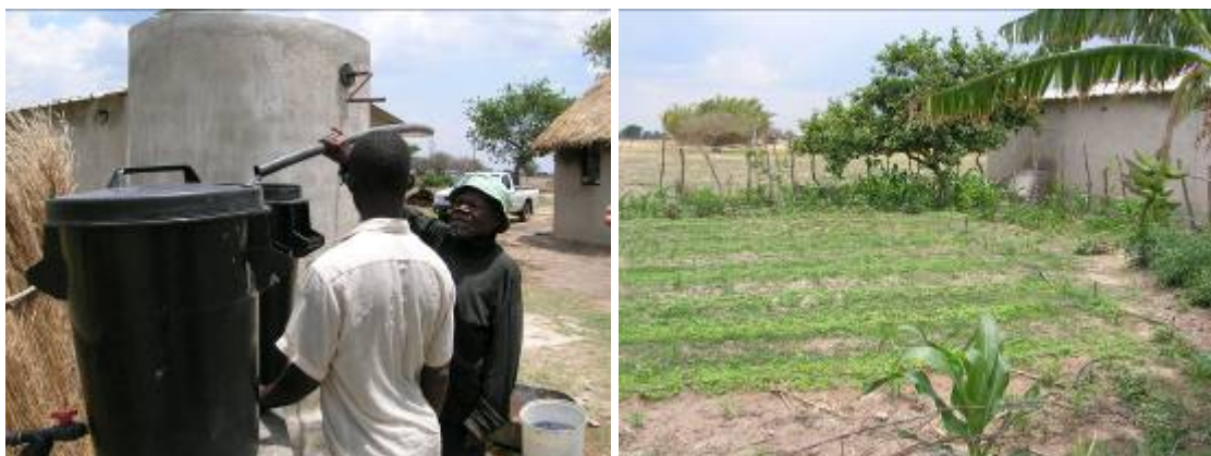
Figure 13: Drip kits in Marondera districts: water gets pumped into the tanks from the rope pump, and distributed to the plot via the laterals with emitters
