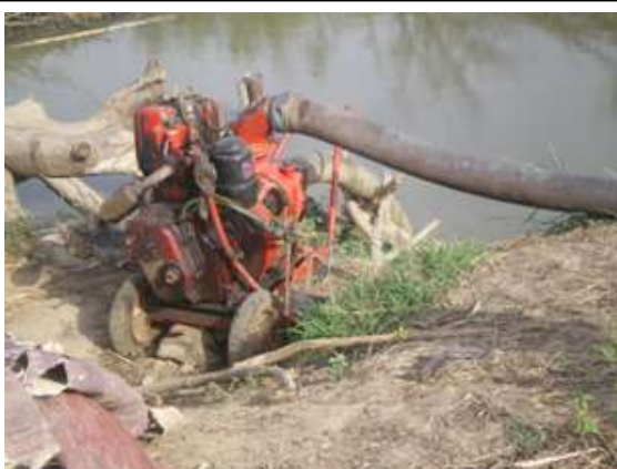
Photo 11: Diesel pump to abstract water from the river. Photo: Eric Ofosu
