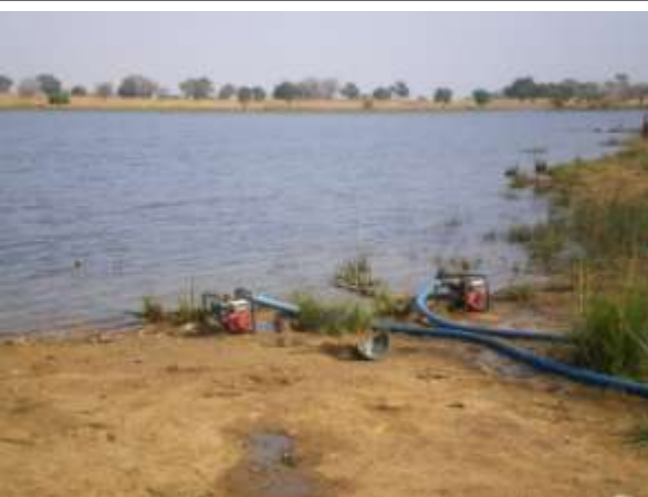
Photo 2: Abstracting water from small reservoir using pumps. Photo: Eric Ofosu
