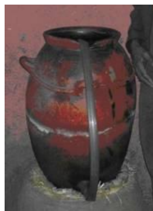
Photograph 8. Home water treatment in locally made earthen pots with a sand filter inside removes 91-99% of bacteria, parasites and turbidity (Guchi 2007). The water is sufficient for daily drinking water requirements, serving a household of 6 people, and a year after introduction, most pots were still used properly in Yubdo-Legebatu, West-Central Ethiopia (Cousins 2007).
