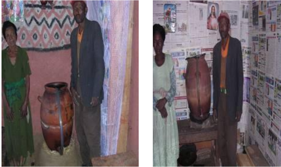
Picture 1. Slow Sand Filtrations in clay pot in two households in Yubudo-Legebatu PAs.
