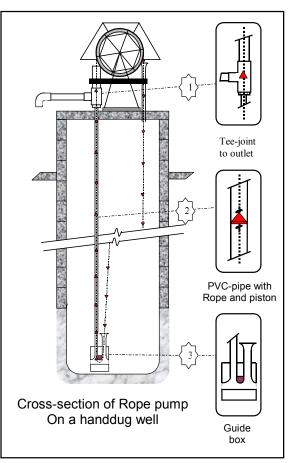
A handdug well should preferably contain at least 1 m of water. In practice the older wells have a depth of about 1 m below the groundwater level of the driest season during the last decades. Of the handdug wells in Nicaragua 45% have a depth of less than 10m; 30% have a depth from 10-20 m; 15% from 20–30 m, and 10% are deeper than 30 m. The maximum depth of handdug wells is about 100 metres although these are only found in exceptional cases.
